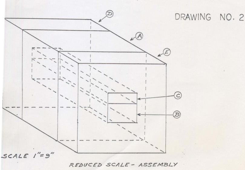
13" IOTES: D AND E OPTIONAL. AN ALTERNATE ARRANGEMENT HAS B AND C OF 13" LENGTH (THE THICKNESS OF A) WITH A YOKE SURROUNDING A AND CONTACTING BOTH ENDS OF B AND C. C. ANOTHER OPTION, WITH B AND C OF 13" AND A ON ITS SIDE, IS TO USE RENTAL TIME ON INDUSTRIAL HYDRAULIC PRESS - AGAINST THE ENDS OF B AND C. 27" 49004674
